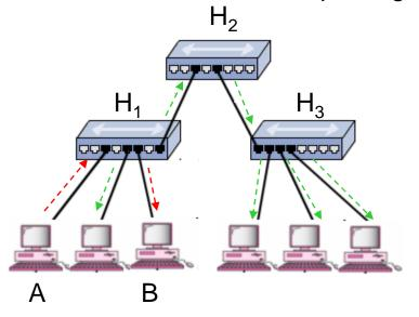
The problem of frame flooding can be resolved by filtering out (not forwarding)<sub>6</sub> frames that have both 'source' and 'destination' address on the same LAN.
