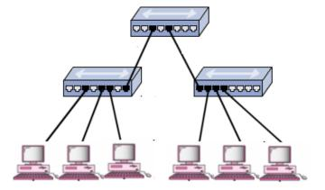
Repeaters and hubs primarily extend the physical reach of a network, but at the same time they can create problems.
