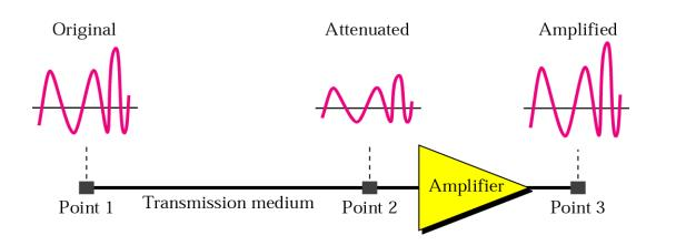
Attenuation : Loss in signal power as it is transferred across a system (medium)
