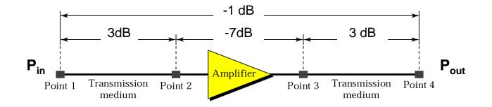
In this case, the attenuation can be calculated as: 3-7+3 = -1, which means that the signal has gained power.
