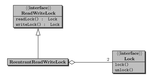
The read-lock is used in the contains method and the write-lock is used in the add method as follows.
