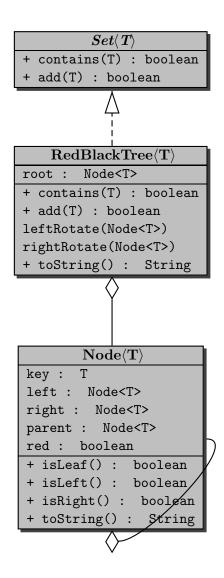
Note that both the RedBlackTree class and the Node class contain a toString method. This method is useful for debugging and testing. The methods leftRotate and rightRotate are auxiliary methods to the add method.
