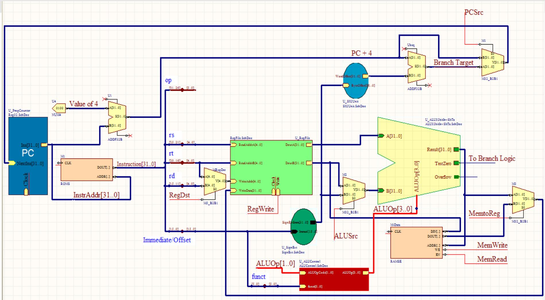
Number of control lines is 11 (4 for MUX's, 4 for ALU control, 2 for data memory, 1 for register file)
