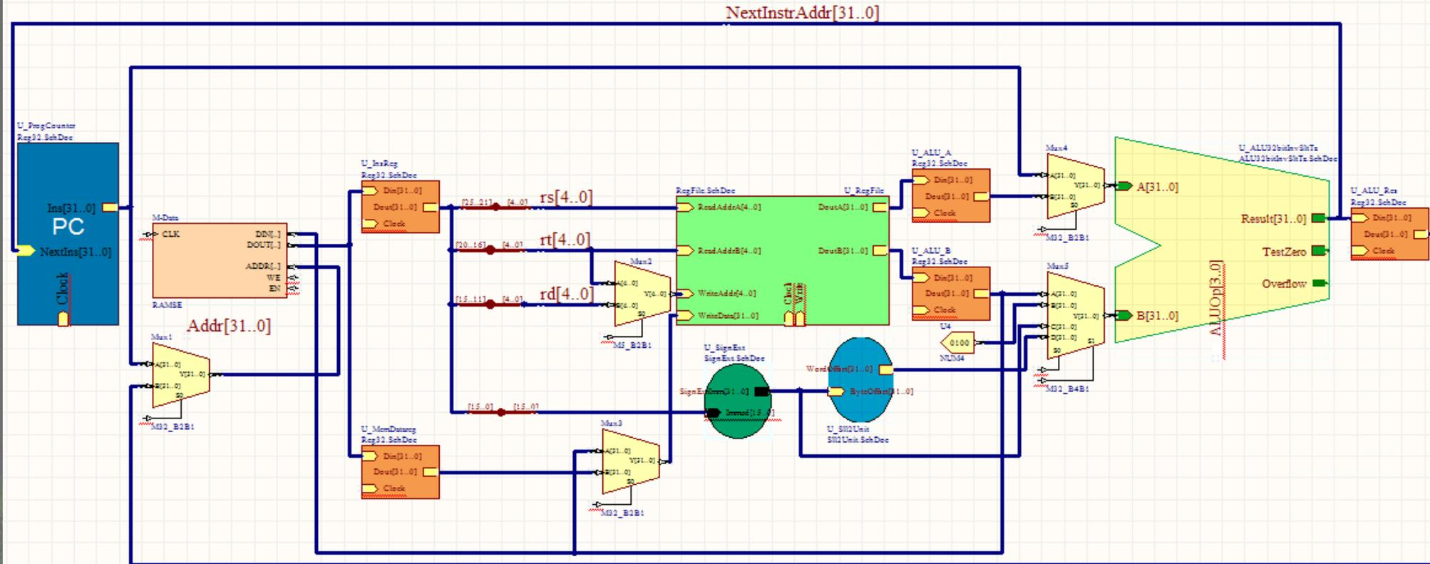
Because functional units are shared, multiplexers are added to select data between different devices
