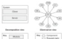
Figure P.5 A client-server system might consist of two modules but eleven components.
