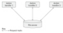
Figure P.4 This system could be in the shared-data style, or the client-server style, depending on your perspective.
