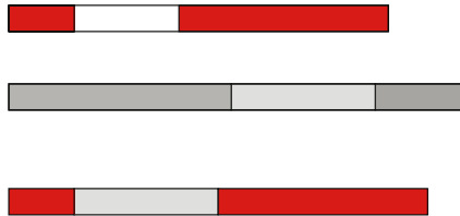
Fig. 12. Typical linear GP crossover. Two instructions are randomly chosen in each parent ( top two genomes ) as cut points. If the code fragment excised from the first parent is replaced with the code fragment excised from the second to give the child ( lower chromosome )
