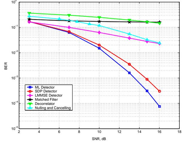
Fig. 2. BER as a function of SNR for different detectors. Simulation parameters: BPSK modulation,  $n = 10$ .
