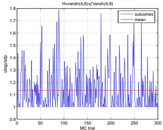
Fig. 3. Upper bound on  $\frac{v_{\text{qp}}}{v_{\text{sdp}}}$  for  $m = 8$ ,  $n = 4$ , over 300 realizations of complex Gaussian i.i.d. channel vector entries.
