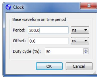
Figure 12. Options available for the Overwrite Clock tool.
