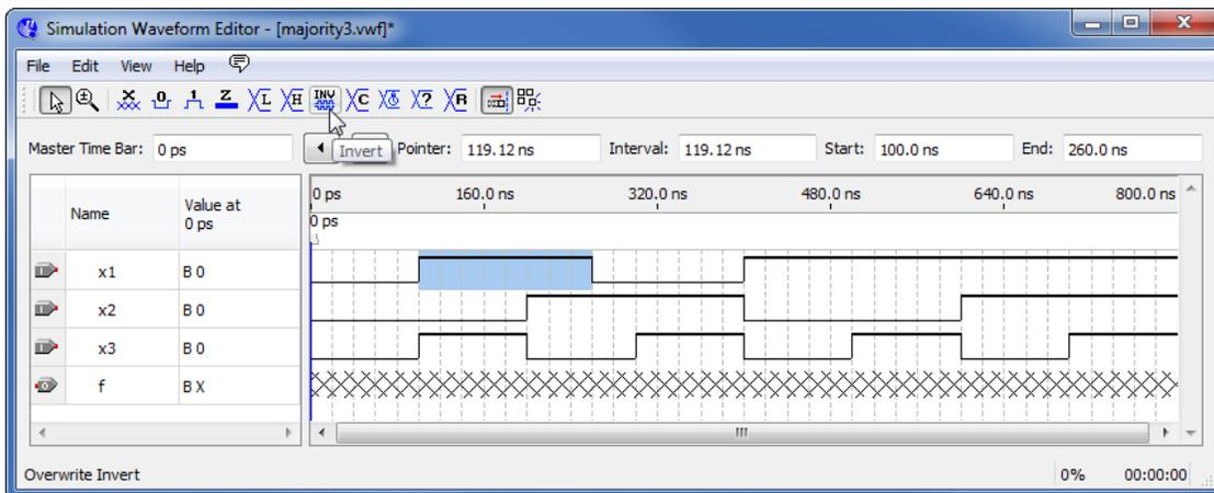
Figure 9. Inverting the *x1* signal from 100 to 260 ns.
