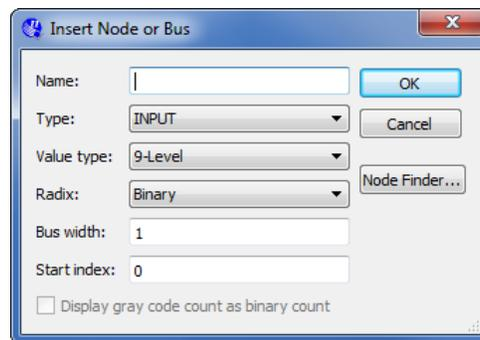
Figure 6. The Insert Node or Bus dialog.
