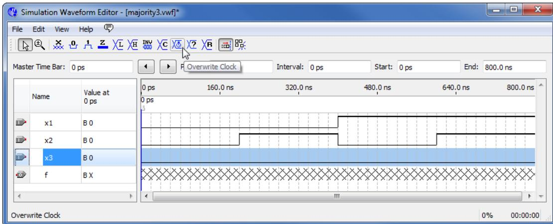
Figure 14. Drawing the waveform for x3.
