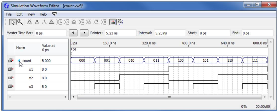
Figure 23. An example of expanding a multibit signal.
