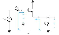
Since there is a resistance RL connected to the source, it is easier to use the T-model
