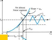
$$g_m = \frac{i_D}{v_{GS}} = k_n \left(\frac{W}{L}\right) (V_{GS} - V_t)$$
