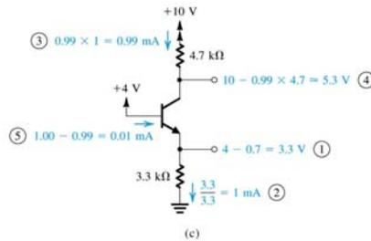
Figure 6.22 Analysis of the circuit for Example 6.4: (a) circuit; (b) circuit redrawn to remind the reader of the convention used in this book to show connections to the power supply; (c) analysis with the steps numbered.
