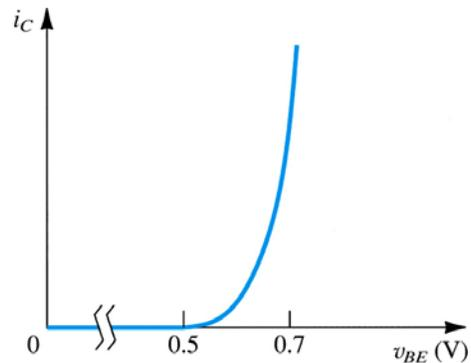
At a constant collector current, the BE voltage decrease by  $-2 \text{ mV}/^\circ\text{C}$
