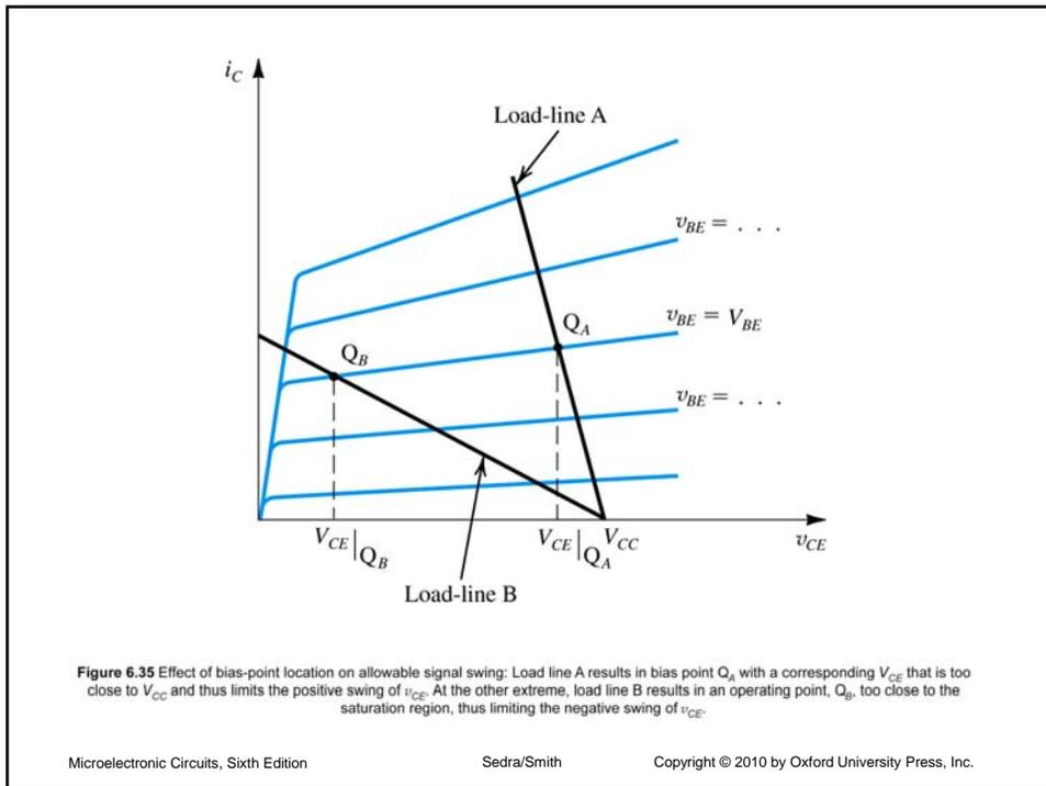
**Figure 6.35** Effect of bias-point location on allowable signal swing: Load line A results in bias point  $Q_A$  with a corresponding  $V_{CE}$  that is too close to  $V_{CC}$  and thus limits the positive swing of  $v_{CE}$ . At the other extreme, load line B results in an operating point,  $Q_B$ , too close to the saturation region, thus limiting the negative swing of  $v_{CE}$ .
