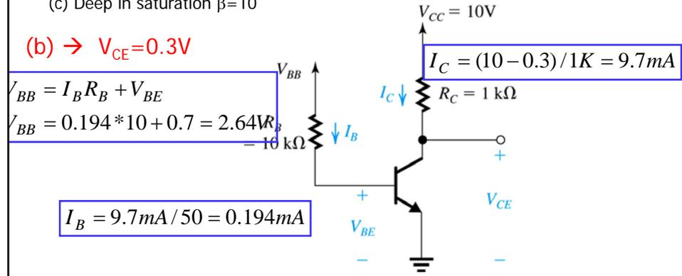
Figure 6.21 Circuit for Example 6.3.
