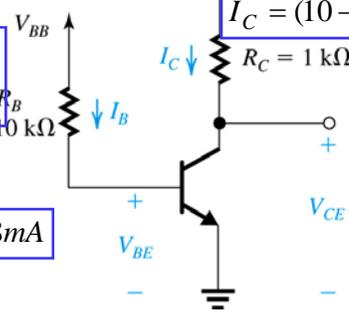
Figure 6.21 Circuit for Example 6.3.
