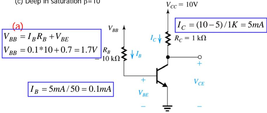
Figure 6.21 Circuit for Example 6.3.
