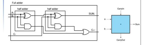
Note: A full adder adds 3 bits. Can also consider as first adding first two and then the result with the carry
