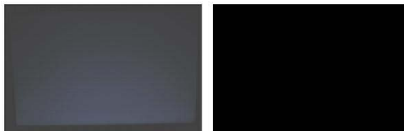
Fig. 5. Left image shows the light leakage symptom in LCD at 0% IRE.
