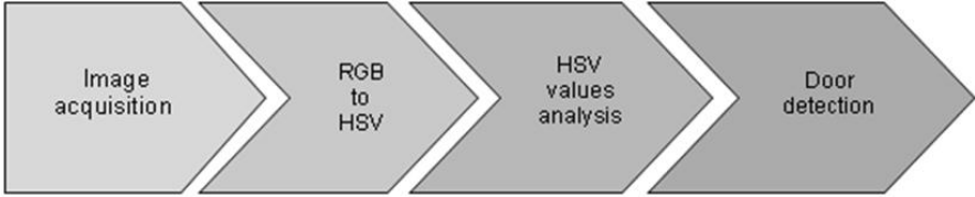
Fig. 7. A block diagram of the process for door detection.
