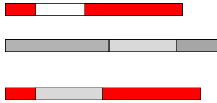
Figure 12: Typical linear GP crossover. Two instructions are randomly chosen in each parent (top two genomes) as cut points. If the code fragment excised from the first parent is replaced with the code fragment excised from the second to give the child (lower chromosome).
