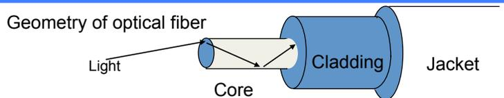
Total Internal Reflection in optical fiber
