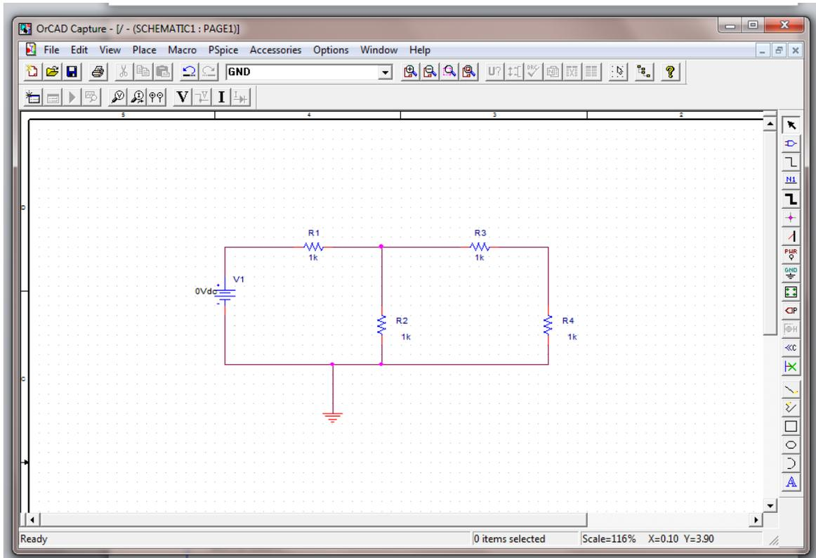
Note that the value of the voltage source is 0V, all the resistors have a value of 1 K $\Omega$ . The names of the resistors are automatically numbered R1, R2, ...
