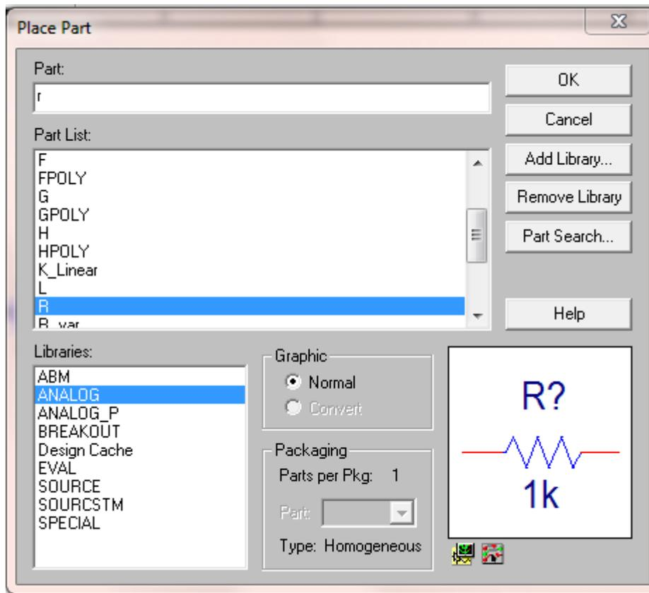
Click 4 times in the schematic to place 4 resistors
