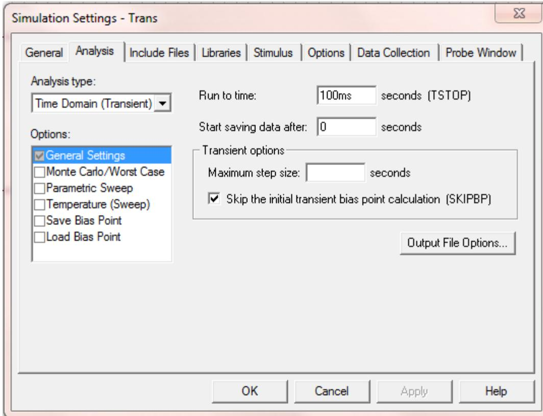
In the Analysis tab choose analysis type to be Time domain (transient), general setting. Choose the run to time 100 msec. (the time constant in the circuit is 20 ms, we will run it five times that). Also start saving data after set it to 0.
