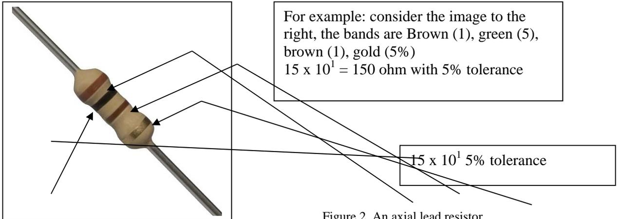
Figure 2. An axial lead resistor
