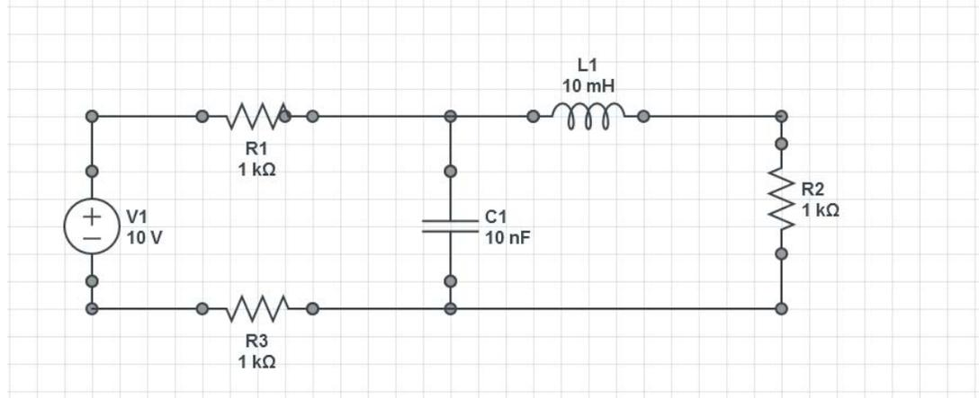
Simulate the circuit displaying the current in the resistor  $R_2$  as a function of time. Choose the time to show the complete behaviour of the current in  $R_2$ .
