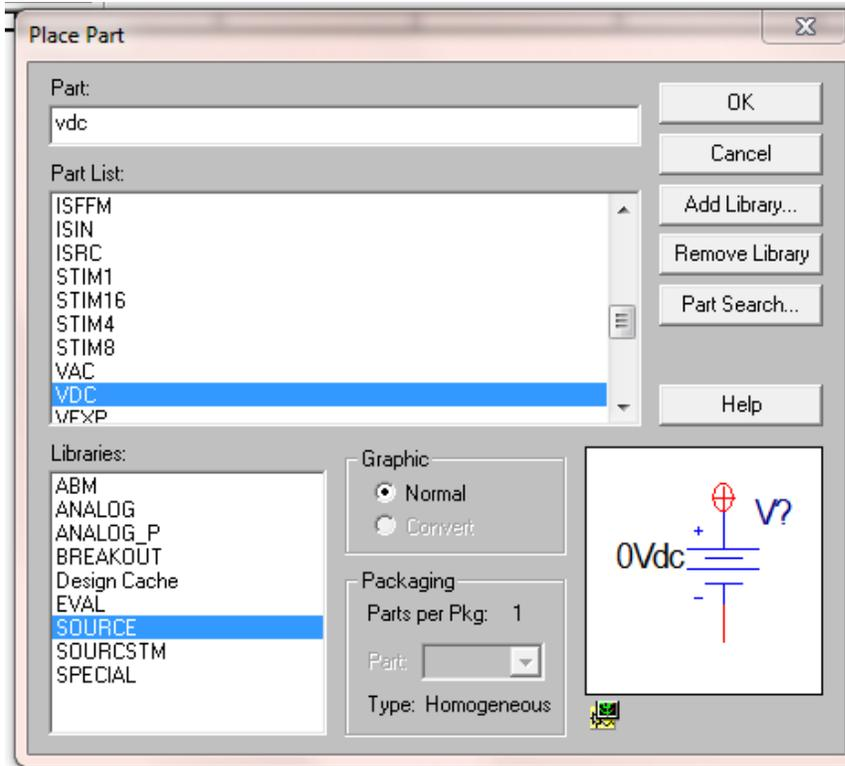
After you chose VDC click O.K (or double click on the part name). The window disappears and the symbol appears attached to the mouse cursor. Go anywhere in the schematic and left click, a copy will be inserted. After that the part still attached to the mouse cursor and you can insert more DC power supplies if you want. We just need one, so right click on the mouse and choose end mode (or hit the Esc key). Highlight ANALOG library and type r in part, the following window appear.
