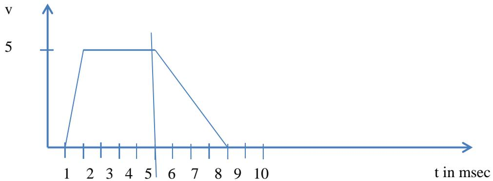
The above waveform is piece linear waveform. It stays at 0 V till 1 msec. Then it, goes linearly from 0 to 5 V for another millisecond. Stays at 5 V for 4 msec. then it goes linearly to 0 in 4 msec.
