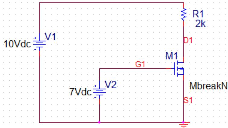
The only new thing here is the MbreakN. In Spice a device starts with M is a MOSFET transistor. From the Breakout library choose “MbreakN 3”. Use net alias to name the three nodes of the MOSFET to G1 (gate) S1 (source) and D1 (drain).
