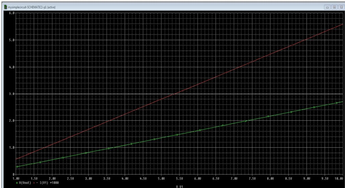
The plot shows two graphs, the green one is  $V_{out}$  and the red one is  $I[V1]$ .
