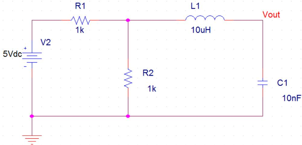
Plot  $V_{out}$  vs. time. Choose the time scale to show the transient response of the circuit. For the values shown, you should not get overshoots. (not underdamped). Change the value of the capacitor to get a reasonable underdamping. What is the value you choose? Plot  $V_{out}$  vs. time to show the step response. How long did it take  $V_{out}$  to reach 90% of its steady state value?
