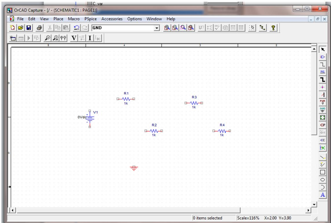
Click on R2, then CTL-R to rotate the resistor into the vertical position. Repeat the same for R4. You can also right click on the resistor and choose rotate.
