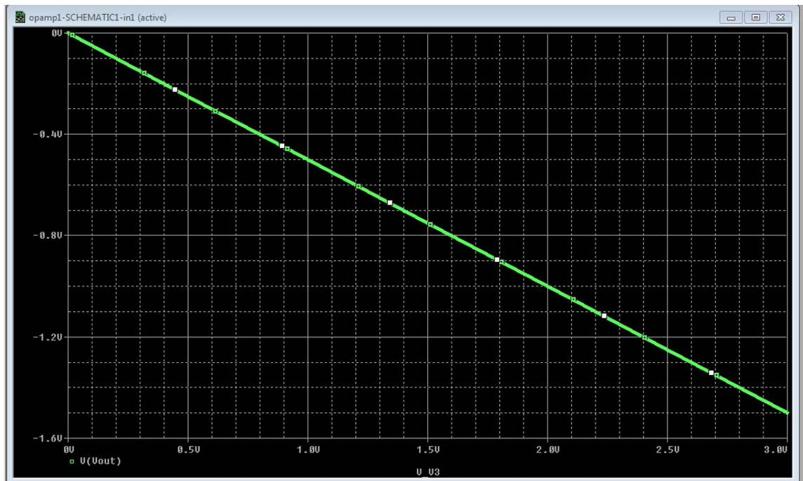
You can see clearly that  $V_{out} = -0.5V_{in}$  as expected for an inverting amplifier configuration.
