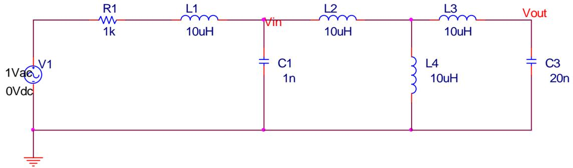
Simulate this circuit showing  $V_{out}$  and  $V_{in}$  as a function of frequency (consider the range from 10Hz to 50MHz).
