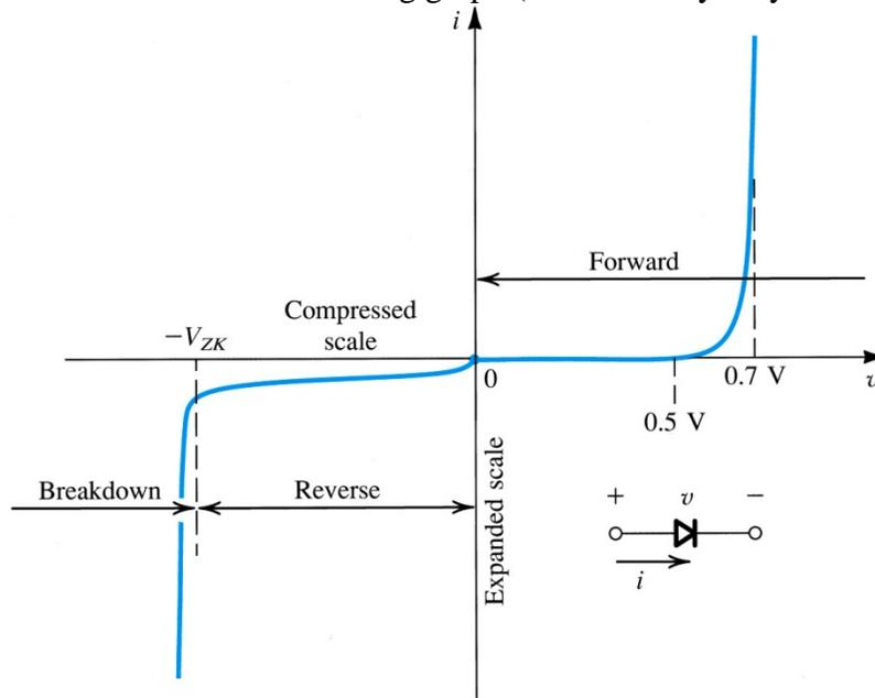
We would like to measure the i-v characteristics of the diode; we will do this in two different ways. First, we construct a simple circuit that allows us to measure the current for different values of the voltage across the diode and plot them. Second, we will use the scope to display the i-v characteristics of the diode.
