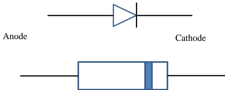
The diode allows current to flow in only one direction (usually, since in the breakdown region the current can flow in the opposite direction). Typically the  $i$ - $v$  characteristics of a diode look like the following graph (numbers may vary from diode to diode).
