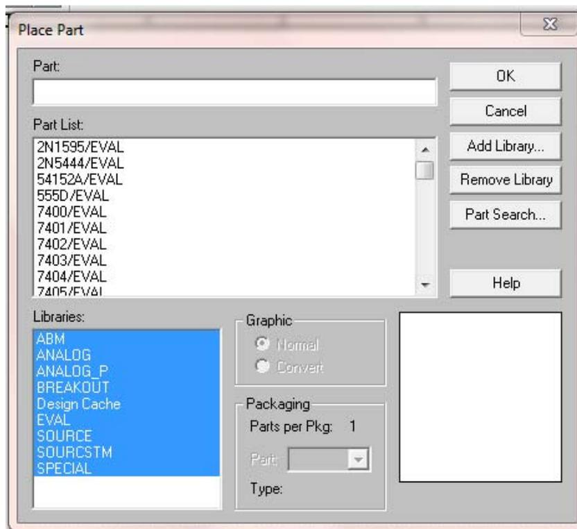
Highlight Source library and write Vdc in “part”. As soon as you right V, all parts that start with V appears, Choose Vdc (A DC power supply) as shown below.
