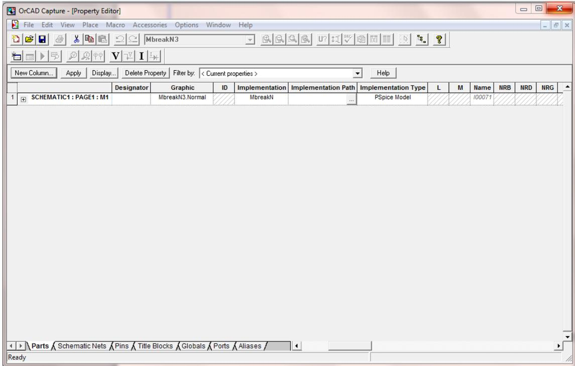
Now, we will edit the SPICE model of our transistor. Highlight the transistor. Highligh the transistor, from the top menu choose Edit → Pspice Model
