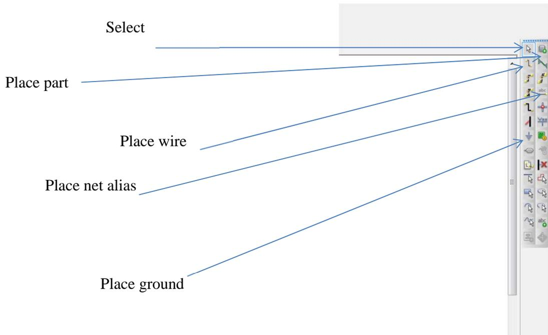
On the right there is a group of fast access keys, the most important is the place part (could also be accessed from the menu bar Place → part. The place ground button (ground is also a part you can access it from the place part button or menu. The place wire (also from the menu Place → Wire). Place net alias (also from the place menu, and the place ground as shown in the expanded figure
