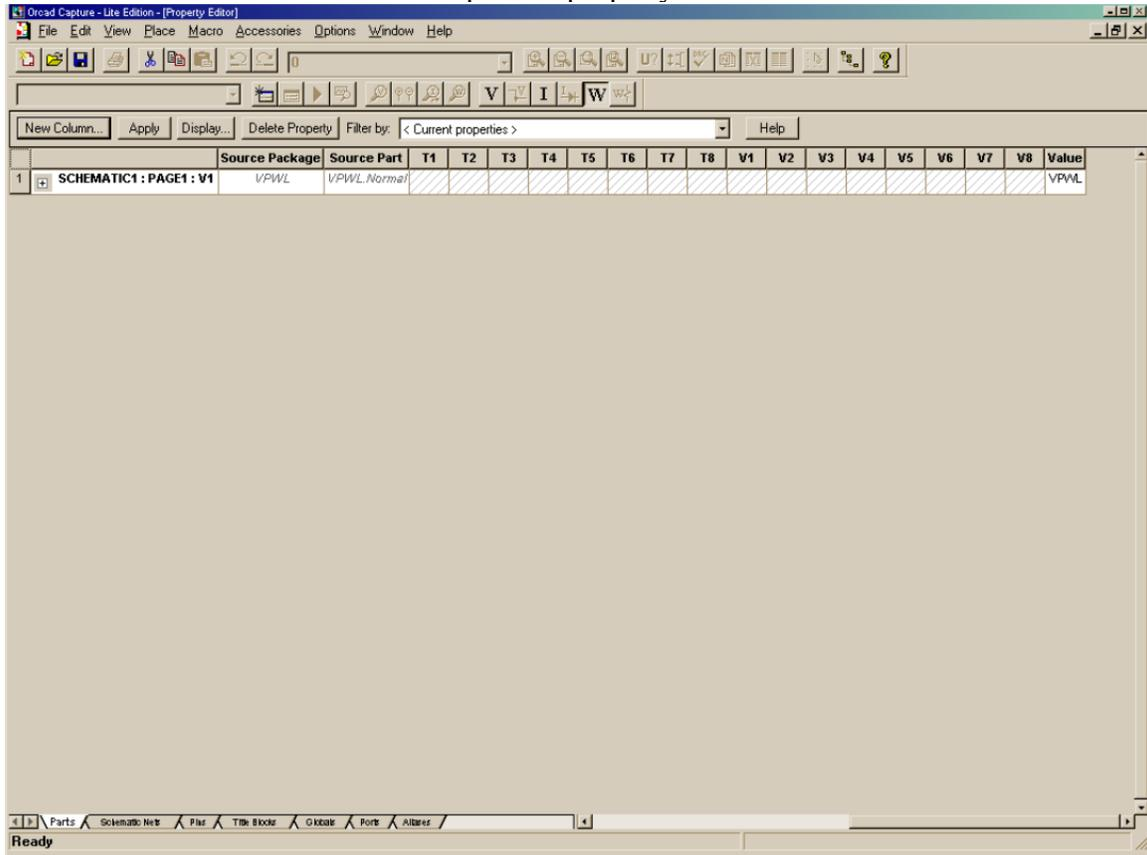
In the Parts tab (bottom part of the window) start inserting columns. Insert columns with the following names and values
