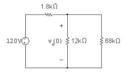
$$R_{\rm eq} = 12 \, \text{k} \| 8 \, \text{k} = 10.2 \, \text{k} \Omega$$
