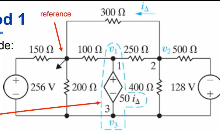
$$\frac{v_1}{100} + \frac{v_3}{200} + \frac{v_3 + 256}{150} + \frac{v_1 - v_2}{250} + \frac{v_3 - v_2}{400} + \frac{v_3 - 128 - v_2}{500} = 0$$
