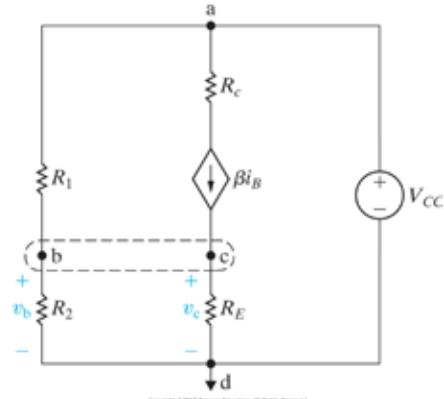
$$\frac{v_b - V_{CC}}{R_1} + \frac{v_b}{R_2} + \frac{v_c}{R_E} - \beta i_B = 0$$
