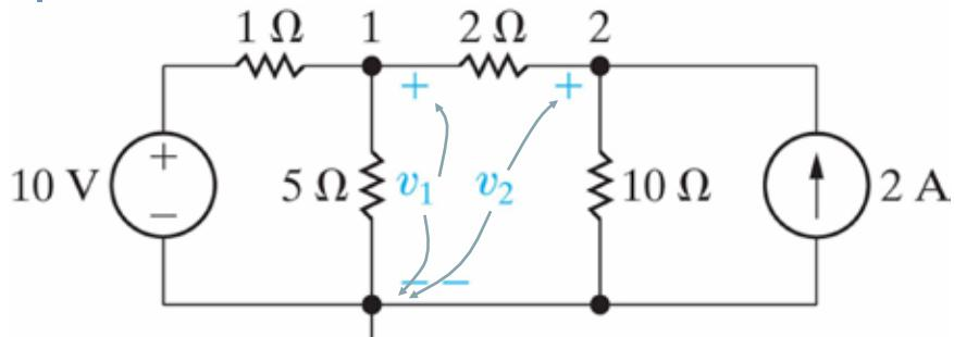
$$-\frac{10 - v_1}{1} + \frac{v_1}{5} + \frac{v_1 - v_2}{2} = 0 \quad -\frac{v_1 - v_2}{2} + \frac{v_2}{10} - 2 = 0$$
