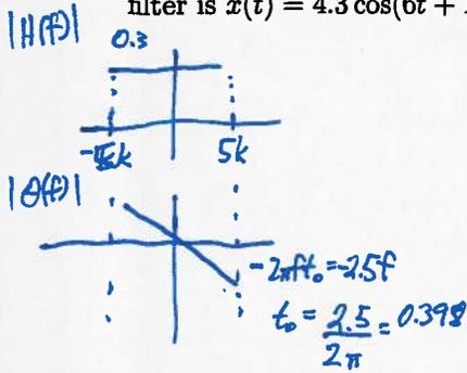
$$\begin{aligned} \therefore y(t) &= 0.3 \times 4.3 \cos(6[t - 0.398] + 12^\circ) \\ &= 1.29 \cos(6[t - 0.398] + 12^\circ) \\ &= 1.29 \cos(6t - 124.78^\circ) \end{aligned}$$
