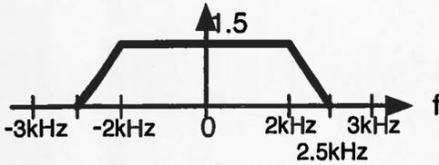
$$\begin{aligned} W_n \times G_x(0) &= P_x \\ W_n \times 1.5 &= 1.5 \times 2 + \frac{1.5 \times 0.5}{2} \\ W_n &= 2 + \frac{1}{4} = 2.25 \text{ kHz} \end{aligned}$$
