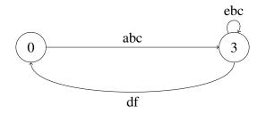
Marking scheme: 1 mark for state 0, 1 marks for state 3, 1 mark for transition labelled abc from 0 to 3, 1 mark for transition labelled ebc from 3 to 3, 1 mark for transition labelled df from 3 to 0
