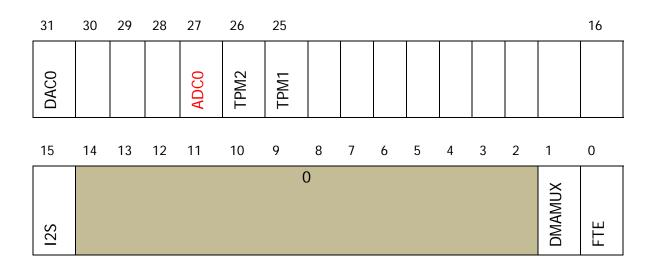
In order to enable the clock to the ADC0 module, set bit 27 (ADC0) to 1.
