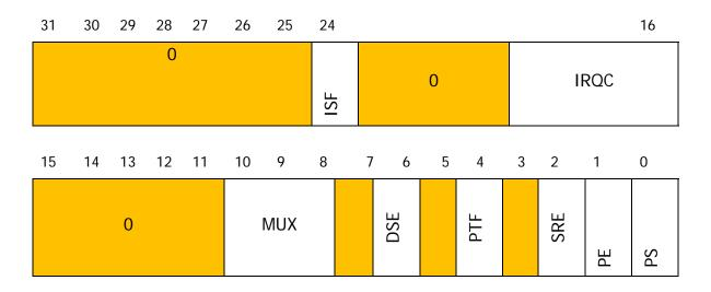
ISF if configured for interrupt, 0 -> interrupt not detected, 1-> detected writing 1 clears the flag
