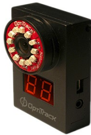
Figure 1 - NaturalPoint OptiTrack FLEX C120 Camera
