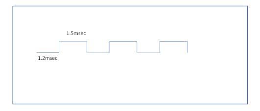
In the square wave shown above, the LOW time is 1.2 msec, and the HIGH part is 1.5 msec. The total cycle time is 2.7 msec. which means the frequency of the PWM is 1/2.7msec = 0.37 KHz or 370 Hz. The duty cycle of the wave is 1.5/2.7 = 55.5%
