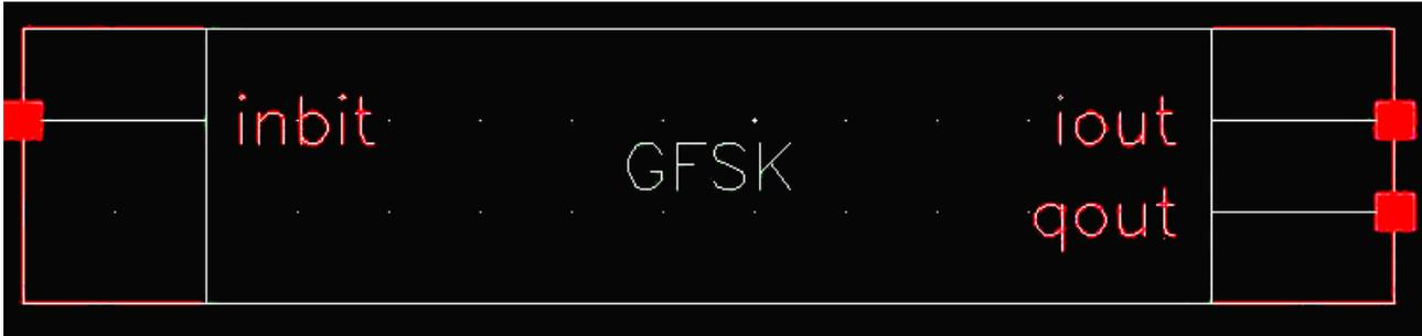
GFSK is a Gaussian filtered frequency modulation I and Q signal generator, which makes the I and Q output smoother so as to limit the spectral width. GFSK is poorer in terms of the spectral efficiency but easier to implement as compared to GMSK. GFSK is often seen in cordless phones using the DECT standard and in bluetooth.
