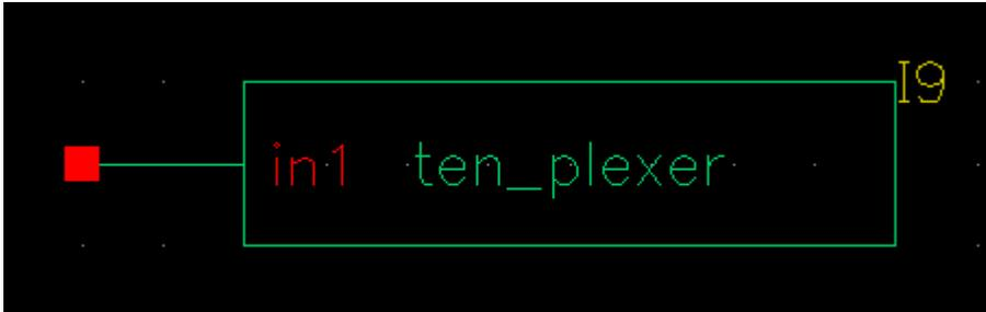
The `ten_plexer` is a series of ten Bessel filters followed by ten `portAdapters` and ten ports. Bessel filters are chosen because there is no ripple in the passband of the filter and the transient response is not complicated. This allows a `tstab` to be set in the simulation to allow the filters to reach steady-state.
