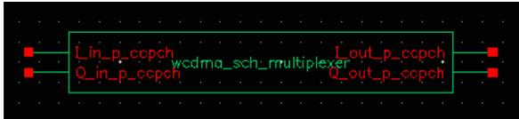
This module produces the synchronization channel and performs SCH multiplexing. The parameters of the module are:
