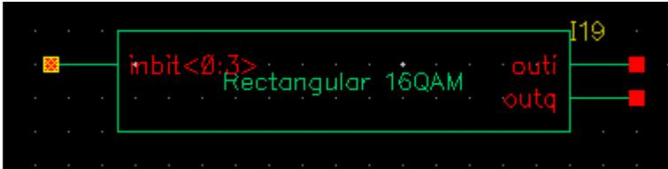
Rectangular\_16\_QAM takes in a bit signal or generates a pseudo-random bit stream internally and then generates an unfiltered I and Q modulating signal at the output. The number of QAM states is 16 and the output is generated as 16-QAM points separated by the voltages specified by the Dist\_or\_power property by default.
