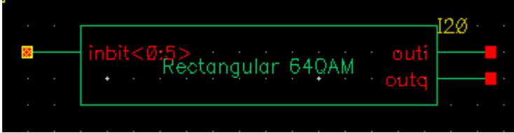
Rectangular\_64\_QAM takes in a bit signal or generates a pseudo-random bit stream internally and then generates an unfiltered I and Q modulating signal at the output. The number of QAM states is 64 and the output is generated as 64-QAM points separated by the voltages specified by the `Dist_or_power` property by default.
