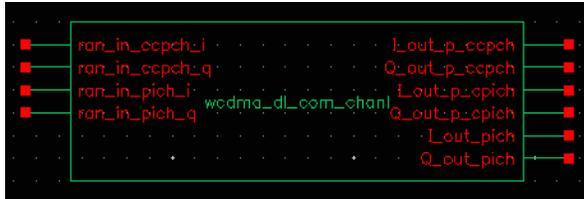
This module, with four inputs and six outputs, generates the pCPICH (primary common pilot), PICH (paging indicator channel) and pCCPCH (primary common control physical channel). For PICH and pCCPCH, either external or internal random signals can be selected according to the value of the `enable_input` parameter. The parameters of the module are:
