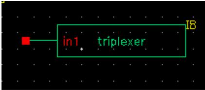
The `triplexer` is a series of three Bessel filters followed by three `portAdapters` and three ports. Bessel filters are chosen because there is no ripple in the passband of the filter and the transient response is not complicated. This allows a `tstab` to be set in the simulation to allow the filters to reach steady-state.
