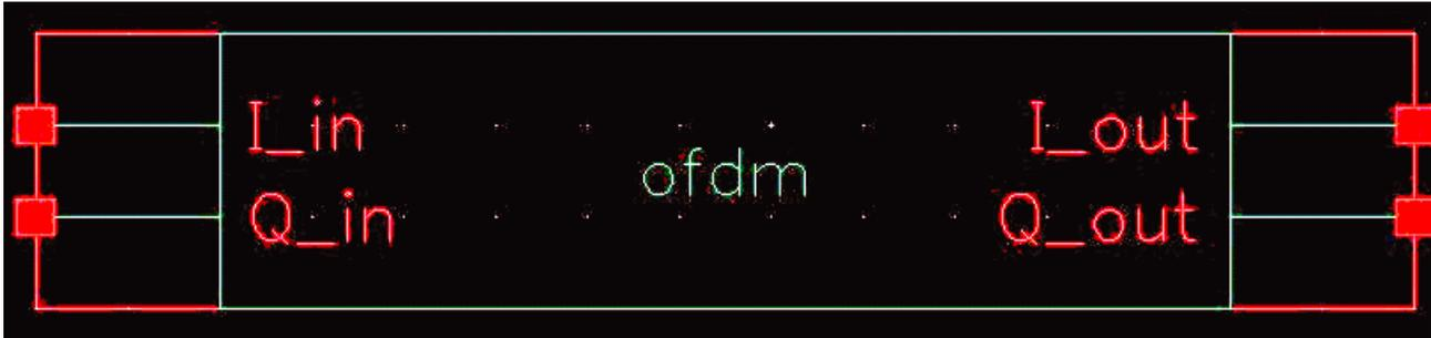
OFDM is a digital multi-carrier modulation scheme, in which closed-spaced sub-carriers are summed into main carrier. These sub-carriers are orthogonal to each other and modulated with conventional modulation scheme at a low symbol rate. The summation is performed through Fast Fourier Transform.
