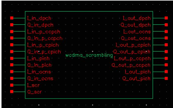
This module scrambles the spread code. The parameters of the `wcdma_scrambling` module are:
