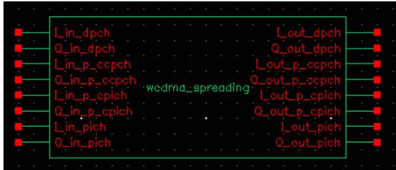
This module spreads the data over the OVFS codes. The parameters of the wcdma\_spreading module are:
