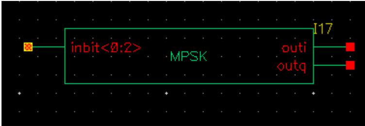
MPSK takes in a bit signal or generates a pseudo-random bit stream internally and then generates an unfiltered I and Q modulating signal at the output. The number of PSK states is eight, and the output is generated as points on a unit circle.
