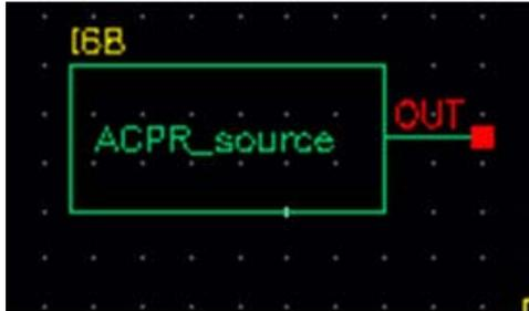
The `ACPR_source` is used to generate modulated RF waveforms. It is a self-contained RF modulator. The out connection is the modulated RF output.
