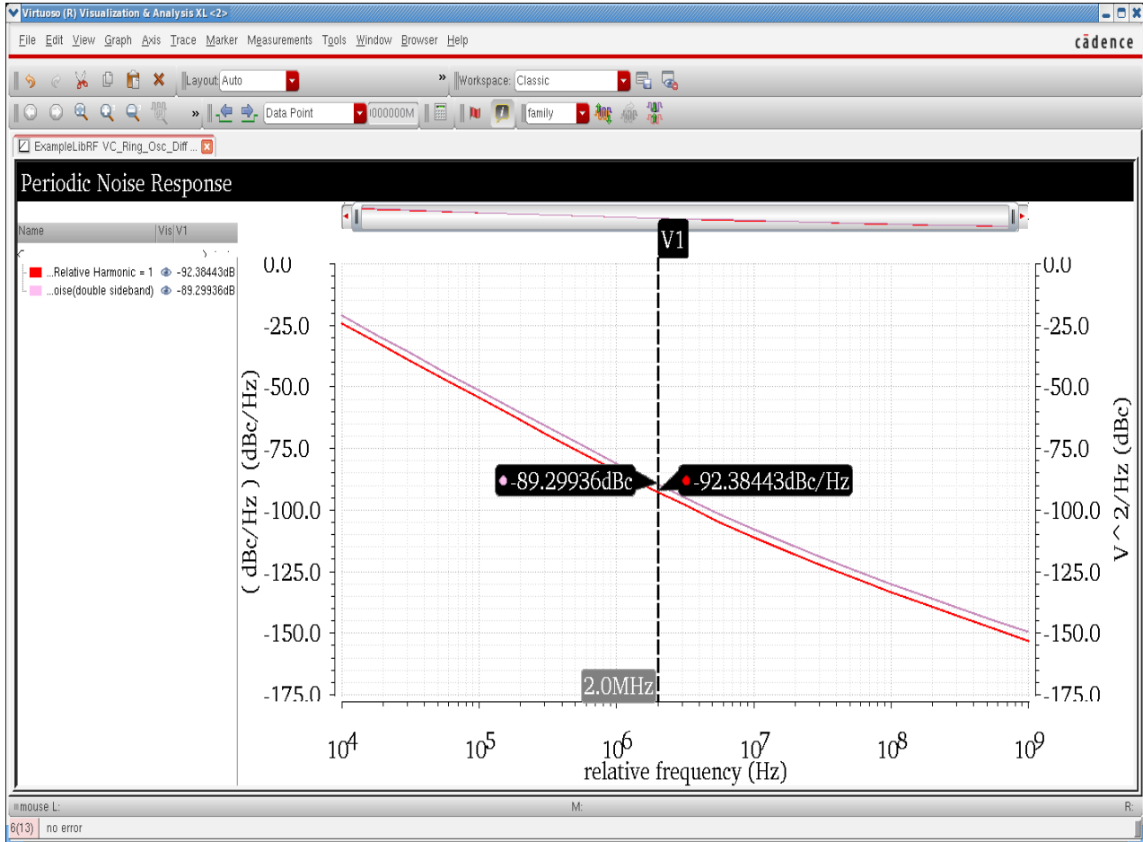
Figure A-267 DSB and SSB phase noise plot showing 3dB difference
