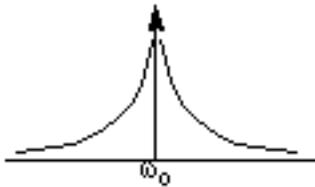
The amplification near the oscillation frequency that generates the phase noise is quantified by assuming the loop gain varies smoothly as a function of frequency in this region [razavi96]. If
